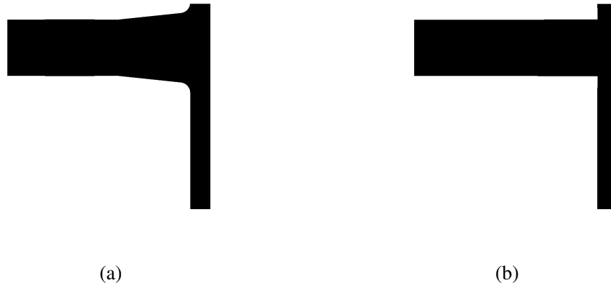
Figure 3.21: Geometry of (a) smooth fitting of experiment and geometry of (b) straight fitting used for sensitivity analyses. Reprinted with permission from [2].
