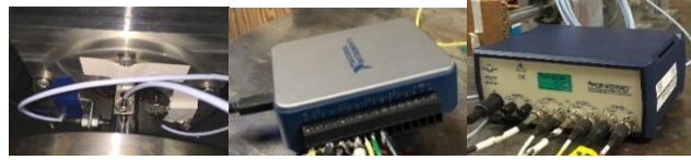
Figure 96. Data acquisition system of the Catcher Bearing test rig. (a) Bently eddy current sensor (b) NI USB DAQ board with 8 channels (c) Load cell signal conditioner
