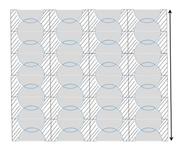
Figure 51. An aggregation of throat unit collectors form the GPF wall.
