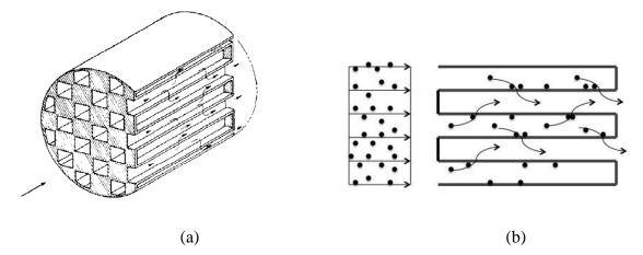
Figure 8. (a) DPF geometry, (b) Illustration of flow through a DPF channel wall.
