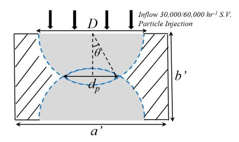
Figure 50. Throat unit collector. *D* is the diameter of cavity;  $d_p$  is pore size; let a' be the side length of the cuboid throat unit collector and b' be the height; angle  $\theta$  changes with the diameter ratio.
