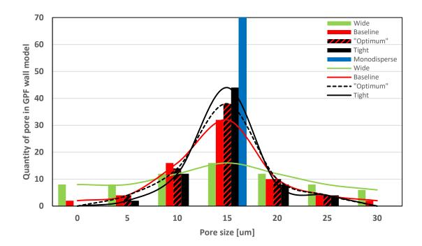
Figure 38. The hypothesized "Optimum pore size distribution" in stacked column graph, next to the baseline, wide, tight and monodisperse distribution. The quantity of each pore size in the "Optimum" distribution is elaborated in Table 4.
