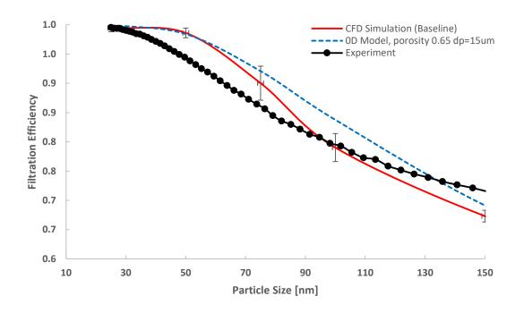
Figure 33. Size-dependent filtration efficiency comparison between the 2-D CFD simulation described in this work, the 0-D model and experiment.
