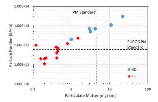
Figure 2. PM and PN emission of GDI engines are higher than PFI engines based on the data from[2].
