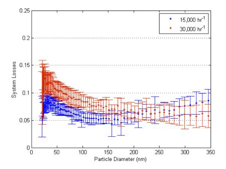
Figure 12. System losses of the empty sample holder.
