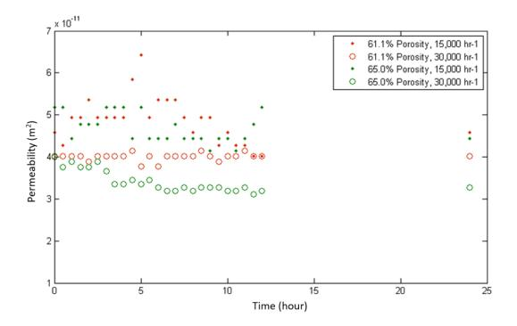
Figure 16. Effect of flowrate on permeability as calculated by the Darcy's Law.
