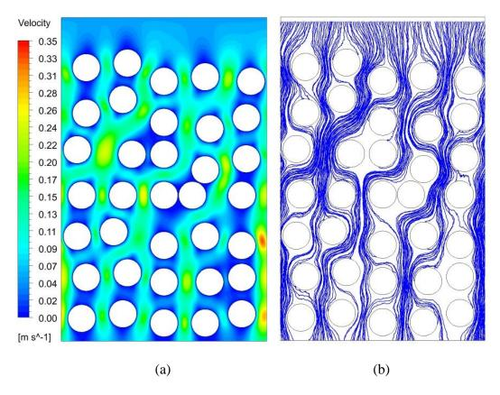
Figure 24. (a) Flow field and (b) particle tracking results of a typical CFD study.
