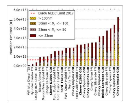
Figure 4. Vehicles PN emission at cold start. Most vehicles at test exceeded EURO 6 PN limit[8].
