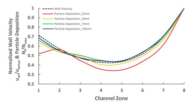
Figure 64. Normalized particle deposition profiles vs normalized wall velocity profile.
