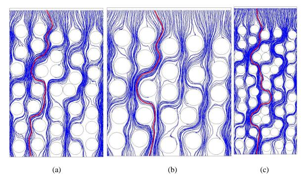
*Figure 43. Particle tracking of (a) baseline, (b) 20um average pore size and (c) 10um average. A streamline is highlighted in red for each case.*
