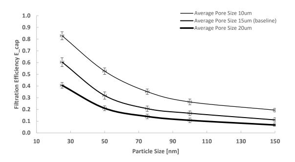
*Figure 41. Size-dependent filtration efficiency with changing average pore size.*
