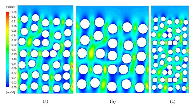
Figure 42. Velocity contour for (a) the baseline, (b) 20um average pore size and (c) 10um average pore size.
