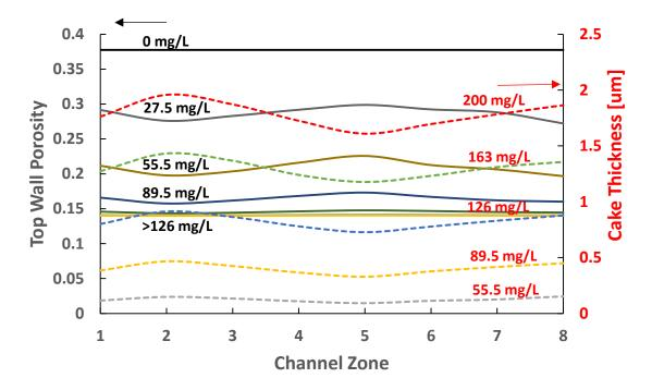
Figure 74. Transient top wall porosity profile and cake distribution.
