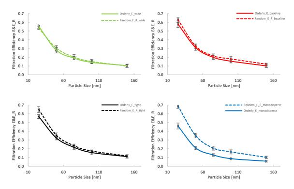
Figure 30. Size-dependent filtration efficiency of random and orderly circular obstacle layout GPF wall model for the baseline, tight, wide and monodisperse pore size distribution.
