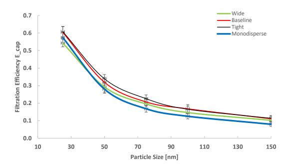
Figure 34. Size-dependent filtration efficiency  $\hat{E}$  for the baseline, tight, wide, and monodisperse pore distributions. For details of the quantities of different pore size for each pore size distribution, please refer to Table 3.
