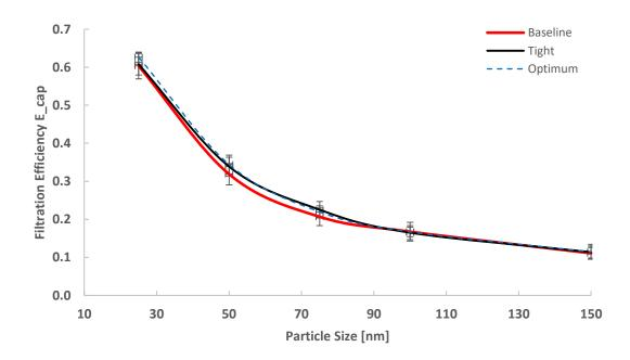
Figure 39. The hypothesized "Optimum pore size distribution" shows similar filtration efficiency with the baseline and tight cases at nearly all particle sizes.
