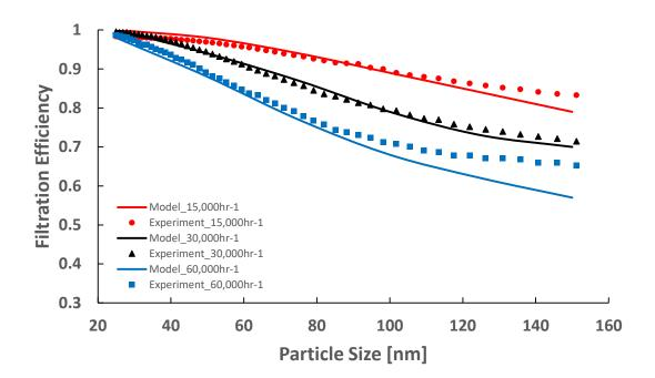
*Figure 68. Model predicted initial filtration efficiency of Blank2, validated by experimental data at 15,000 hr*<sup>-1</sup>, 30,000 hr<sup>-1</sup> and 60,000 hr<sup>-1</sup>.
