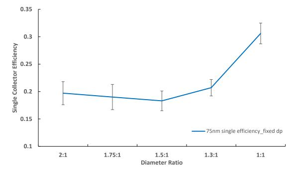
Figure 55. Single collector efficiency changes as diameter ratio decreases. Minimum efficiency is seen at diameter ratio of 1.5.
