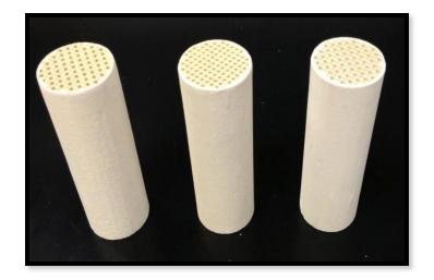
*Figure 10. Cordierite DPF samples. From left to right, the samples have porosities of 55.8%, 61.1% and 65.0%.*
