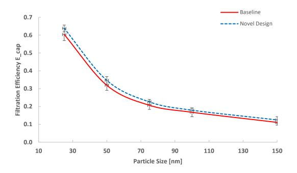
Figure 45. Novel GPF wall design shows increased filtration efficiency as compared to the baseline.
