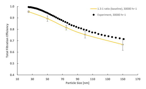
*Figure 54. Total wall filtration efficiency with the baseline diameter ratio throat unit collector, validated by experiment data at 30,000 hr*<sup>-1</sup>.
