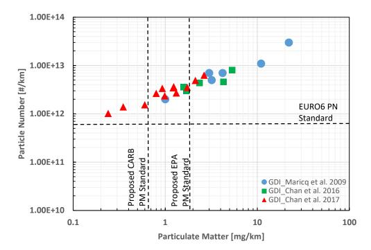
Figure 46. Current GDI engine out particulate emissions exceed EURO 6 and CARB LEV III limit based on data from[2, 59, 60].
