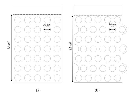
Figure 29. GPF wall models for the same pore size distribution, with (a) orderly obstacle layout and (b) staggered obstacle layout.
