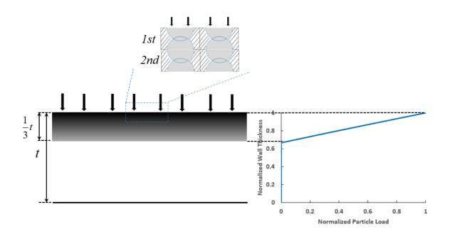
Figure 60. Normalized particle loading profile in the sample GPF wall is assumed to be linear with maximum loading in the first row throat unit collectors. The top rows of throat unit collectors in the zoom view have the same layout as in Figure 51.
