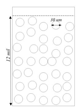
Figure 26. Depiction of the 2-D CFD wall geometry for the baseline pore size distribution.
