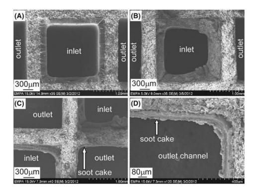
*Figure 6. SEM images of typical DPF soot cake formation at different channel locations. (a) Middle part of DPF (b-c) Inlet part of DPF with thicker soot cake (d) Zoom in image of (c)[12].*
