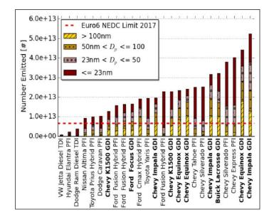
Figure 20. Vehicle PN emissions during cold start[47].
