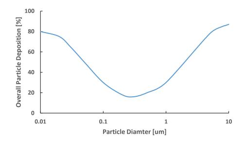
Figure 19. Small size particles, such as GDI PM, have been shown to have high deposition rates in the fine airways, where they can later pass into the blood. The plot is based on data from[5].
