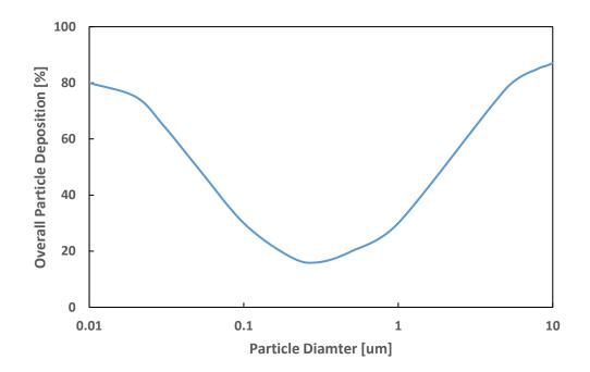
*Figure 3. GDI-sized particles have high deposition rate in fine airway based on data from*[5].
