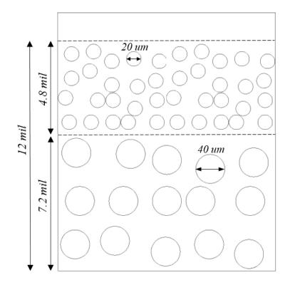
Figure 44. Proposed GPF wall with varying porosity. The top 2/5 of the wall is composed of 10um pores and the bottom 3/5 is composed of 20 um pores.
