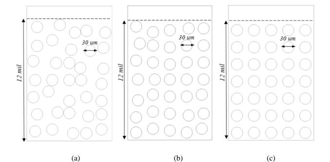
Figure 28. The 2-D CFD wall geometry with (a) wide pore distribution, (b) tight pore distribution and (c) monodisperse pore distribution.
