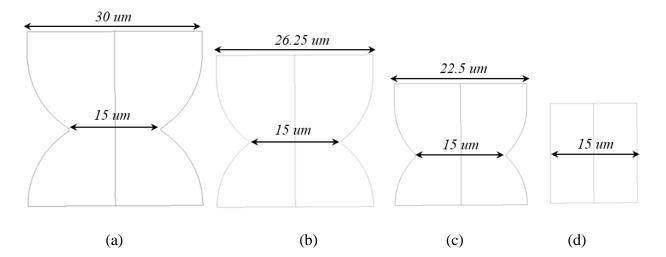
*Figure 53. Throat unit collectors with four different diameter ratio. Diameter ratio (a) 2:1, (b)* 1.75:1, (c) 1.5:1, (d) 1:1.
