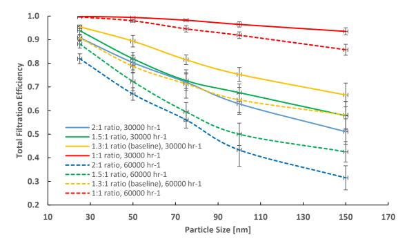
*Figure 56. Total filtration efficiency of throat unit collectors with different diameter ratios, at both 30000 hr*<sup>-1</sup> *and 60000 hr*<sup>-1</sup>.
