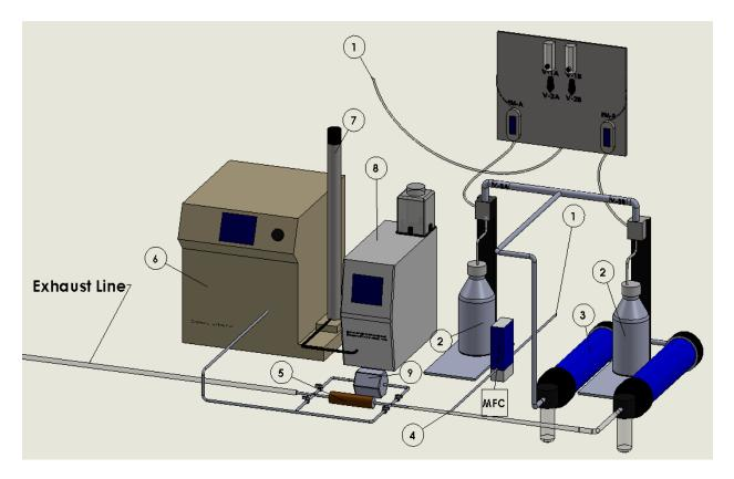
Figure 62. Experiment setup for GPF filtration measurement. (1)HEPA filtered building air is introduced into the system, (2)Atomizers, (3)Gas Dryers, (4)Mass Flow Controller for makeup air, (5)Filter chamber, (6-8)Scanning Mobility Particle Sizer, (9)Differential Pressure Transducer [70].
