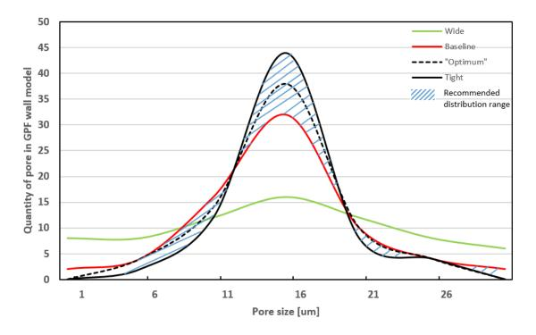
Figure 40. Recommended range of pore size distribution for sample GPF.
