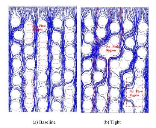
Figure 37. Particle tracking for the (a) baseline and (b) tight pore distributions. Three numbered streamlines shown in red, are singled out to show flow divergence and merging. Regions with low or no flow are marked by red dashed rectangles.
