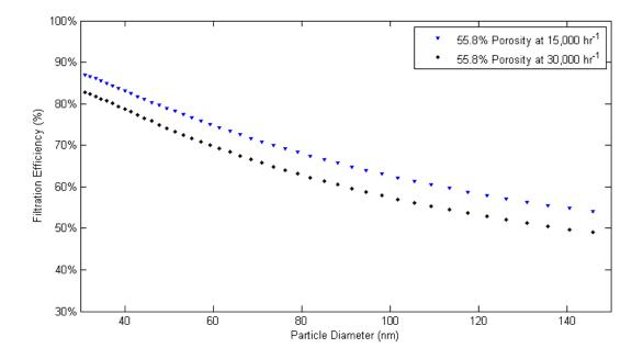
*Figure 15. Comparison of 15,000* hr<sup>-1</sup> and 30,000 hr<sup>-1</sup> filtration efficiencies for a single filter porosity.
