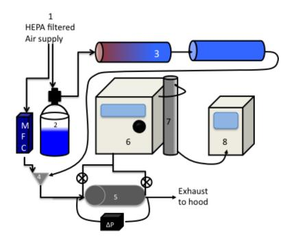
Figure 9. Experimental setup of the filtration and pressure drop characteristic study of filter samples. For each number-labeled devises, (1)Building air supply,(2)Atomizer,(3)Drier,(5)Sample holder,(6-8)SMPS.
