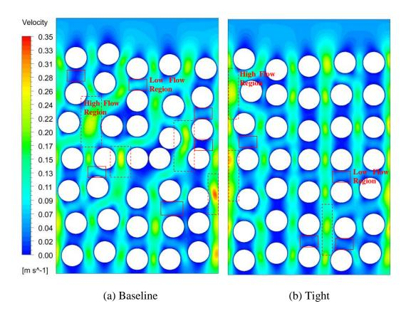
Figure 36. Velocity contours of the (a) baseline and (b) tight pore distributions. High flow velocity regions due to flow merging are marked by red dashed rectangles; Low flow regions resulting from divergence are marked by red solid line rectangular.
