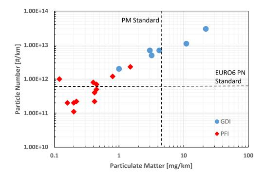
Figure 18. Particulate mass and number emissions from GDI and PFI engines based on the data from[2], with the proposed standards shown by the vertical and horizontal dash lines.
