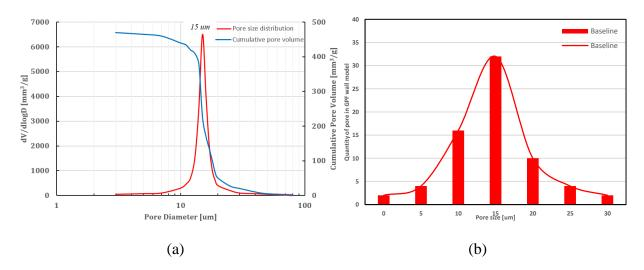
Figure 25. Measure baseline pore size distribution of the sample GPF in (a) logarithmic scale and (b) stacked column graph. The quantity of each pore sized is elaborated in Table 2.
