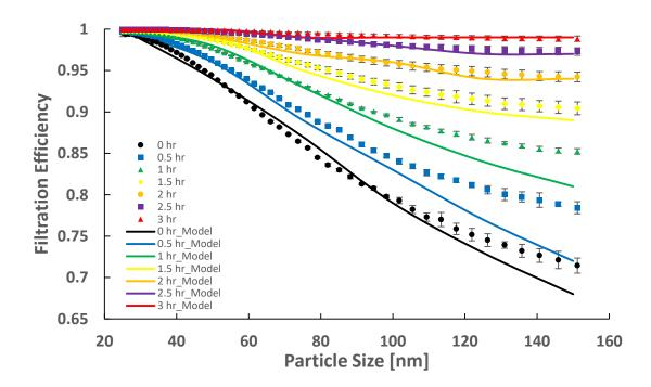
Figure 69. Model predicted transient filtration efficiency of Blank2, validated by experimental data at 30,000  $hr^{-1}$ .
