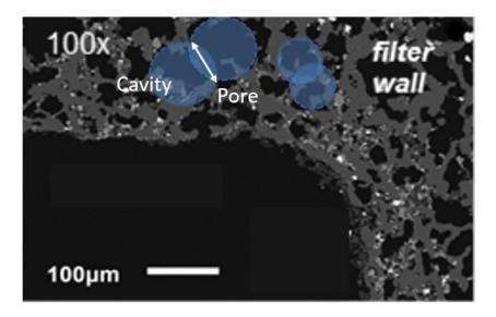
Figure 22. SEM image of a typical GPF wall, showing the cavities and pores microstructure.
