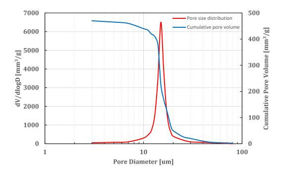
*Figure 21. Sample GPF wall substrate pore size distribution and cumulative pore volume profile based on the mercury porosimetry data.*
