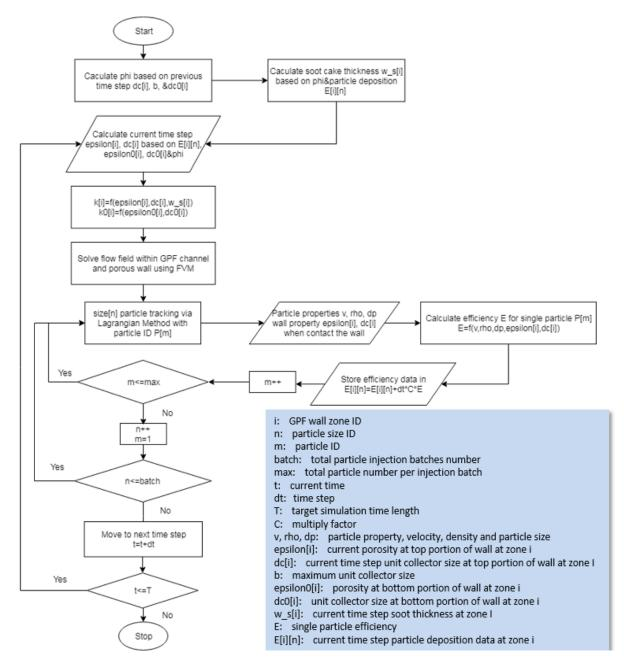
Figure 79. The UDF flowchart demonstrating its functionalities.
