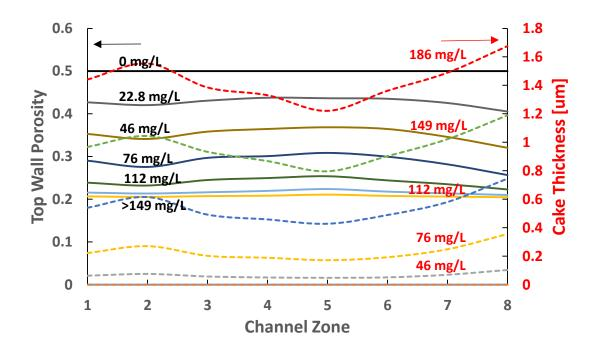
Figure 72. Dynamic top wall porosity profile and cake distribution.
