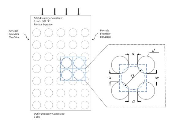
Figure 23. The GPF wall is described by an array of "circular obstacles". The cavities that exhaust flows through are represented by blue dashed lines. Where d is the diameter of the obstacle, a is the horizontal pore spacing; b is the vertical pore spacing, and D is the diameter of the cavity.
