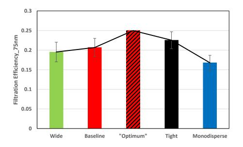
Figure 35. Filtration Efficiency Comparison for 75 nm particles between various pore size distributions in this study indicates the potential existence of an "optimal distribution". For details of the quantities of different pore size for each pore size distribution, please refer to Table 3.
