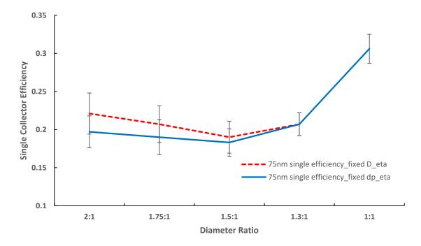
*Figure 58. Single collector efficiency dependency on diameter ratio. Diameter ratio changes either by altering the cavity diameter or pore size.*
