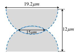
*Figure 52. Schematic of the baseline throat unit collector matching the properties of the sample GPF.*
