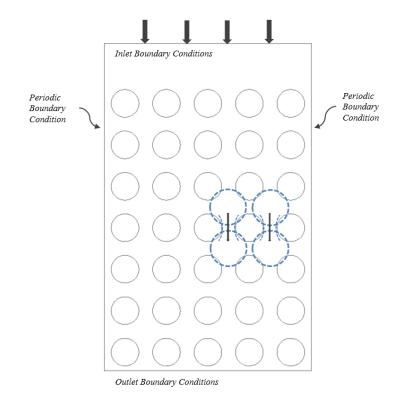
Figure 49. GPF wall model. The cavities that exhaust actually flows through are represented by blue dash line. Let d be the diameter of the obstacle; a is the pore size on horizontal; b is the pore size on vertical; Let D be the diameter of the cavity.
