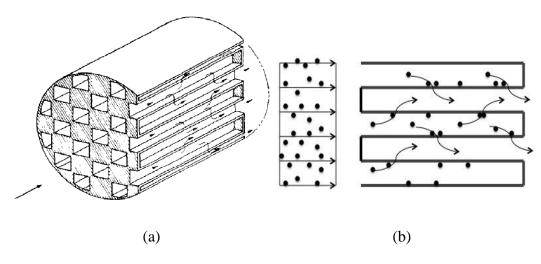
Figure 5. (a) DPF monolith, (b) DPF cross section view showing channel flow inside DPF with particle deposition in and on the porous wall[11].
