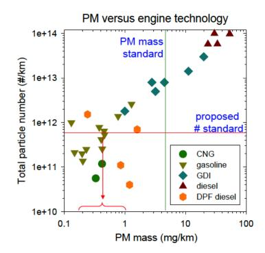
Figure 7. Qualitative differences between particulate emissions of several engine technologies[2].
