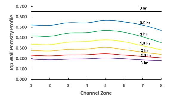
Figure 70. Dynamic top wall porosity profile change with time.
