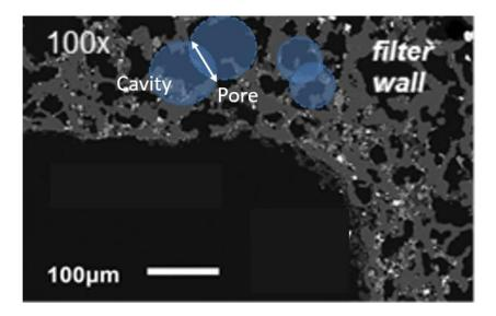
Figure 48. SEM image of a typical GPF wall, showing the cavities, pores and their connectivity.
