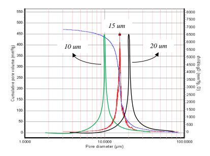
Figure 31. The baseline pore size distribution (a) shifted to right, with average pore size of 20 um; (b) shifted to left, with average pore size of 10 um.
