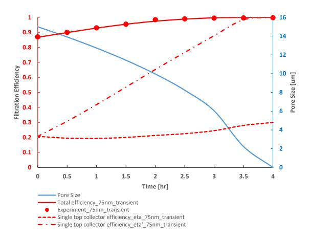
*Figure 61. Model results for transient single collector efficiency, total wall efficiency and experimental results for GPF sample filtration efficiency for 75 nm particles.*
