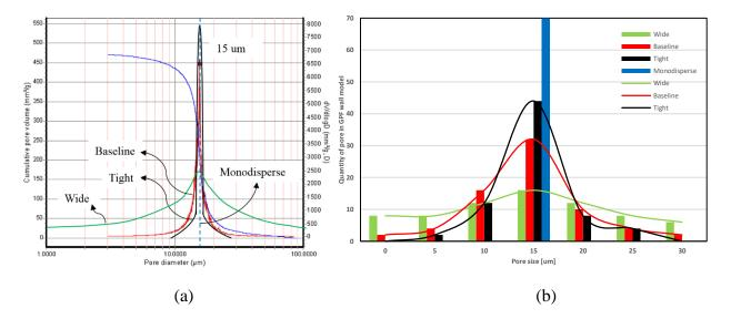
Figure 27. Depiction of the baseline pore size distribution and its wide, tight and monodisperse variations in (a) logarithmic scale and (b) arithmetic scale and stacked column graph. Variance is elaborated in Table 3.
