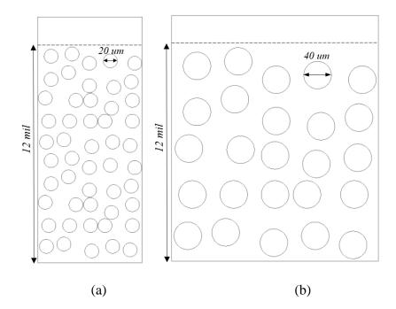
Figure 32. The 2-D CFD wall geometry with baseline pore size distribution (a) shifted to the left, with average pore size of 10 um and (b) shifted to the right, with average pore size of 20 um. The wall thickness and porosity remain unchanged from the baseline condition.
