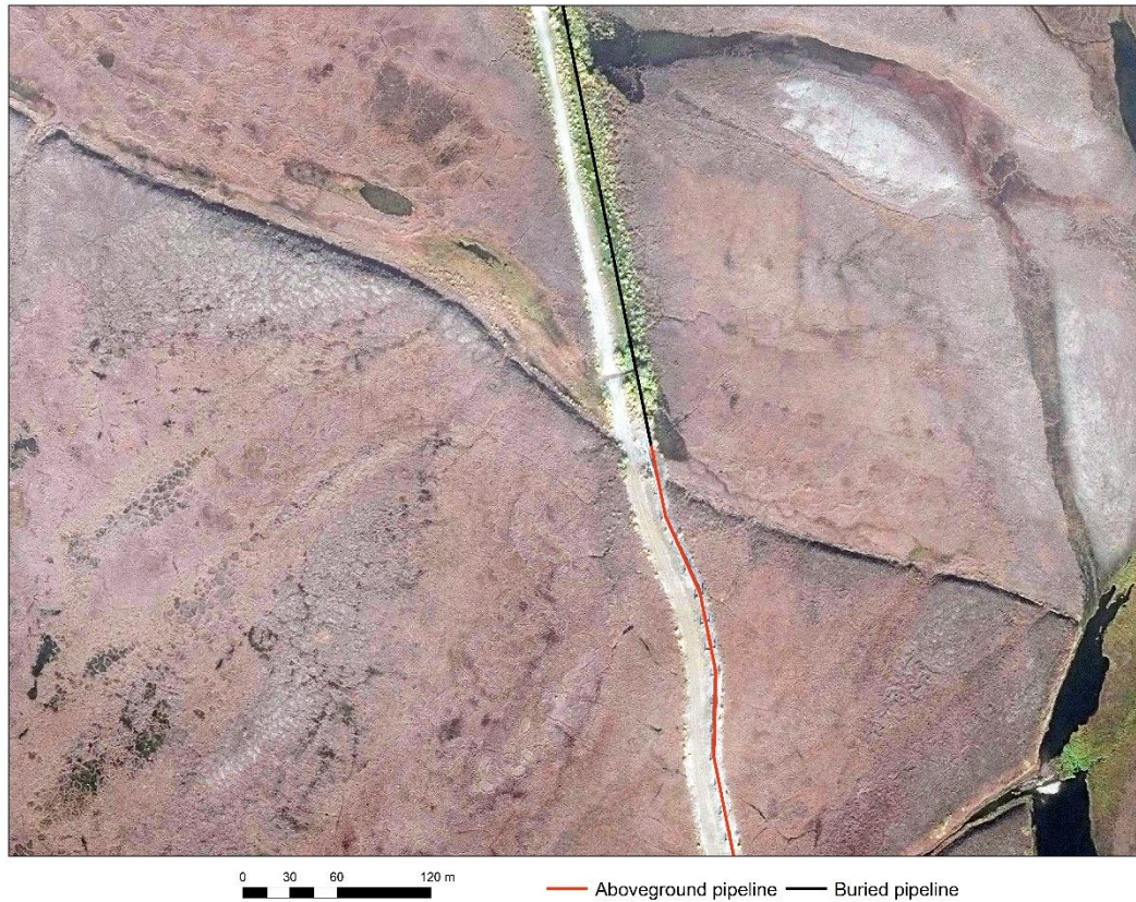
Figure 44: Image from WorldView-3 (© 2016 Digital Globe, Inc.) showing the abrupt change in vegetation along the pipeline as it transitions from aboveground (red) to buried (black). Reprinted from Dwight and Cairns (2018).
