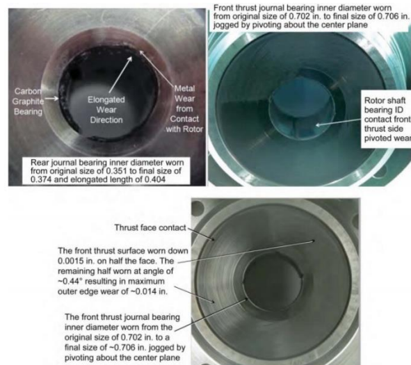
Figure 1-7 Wear pattern in the journal bearings and the thrust bearing
