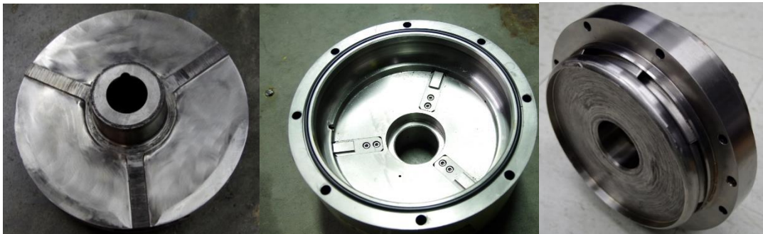
Figure 3-13 The first stage pump impeller with POVs and the inlet casing and the return channel
