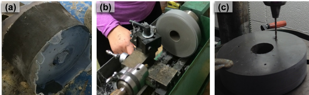
Figure 3.4. Producing Steel/PTFE composite gaskets. (a) Process gaskets using compression molding. (b) Slice and machine gaskets using lathe. (c) Drill holes for thermocouples to pass through the gasket to top and bottom polymer surface.
