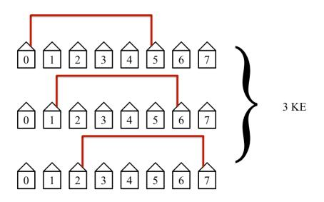
**Figure 12.** The fifth step in the protocol connects the fifth nearest neighbors. This step is not efficient since simultaneous non-overlapping loops with disconnected hosts cannot occur.
