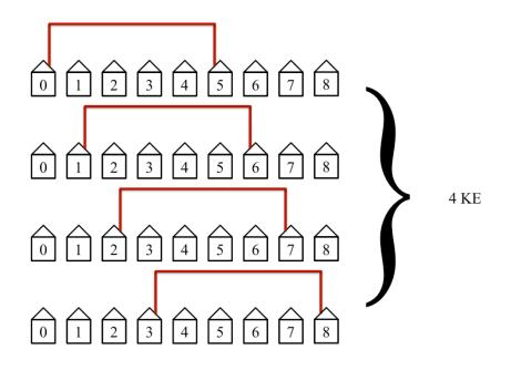
**Figure 19.** The fifth step in the protocol connects the fifth nearest neighbors. This step is not efficient since simultaneous non-overlapping loops with disconnected hosts cannot occur. It requires 4 KEs to complete.
