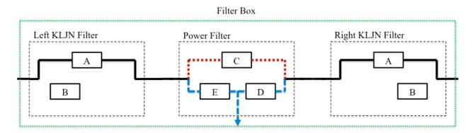
**Figure 6.** The filter box of the inactive host (when it is not executing KLJN key exchange): State 1. Everything is passing between left and right and the host can access only the power. Filter A is passing everything (shorted). Filter B is disconnected. Filter C is passing  $B_{kljn}$  only. Filters and E and D are passing  $f_p$  only.
