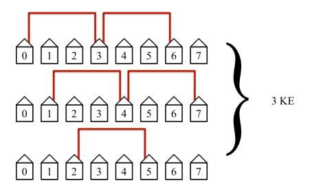
**Figure 10.** The third step in the protocol connects the third nearest neighbors. This step is not as efficient as the first two steps but still has simultaneous loops. This step requires 3 KEs to complete.
