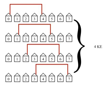
Figure 11. The fourth step in the protocol connects the fourth nearest neighbors. This step is the slowest and least efficient step in the protocol in our example of N=7. This step requires 4 KEs to complete.
