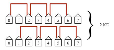
**Figure 9.** The second step in the protocol connects the second nearest neighbors. This step is the second quickest and the second most efficient. It has the second most non-overlapping simultaneous loops and requires 2 KEs to complete.
