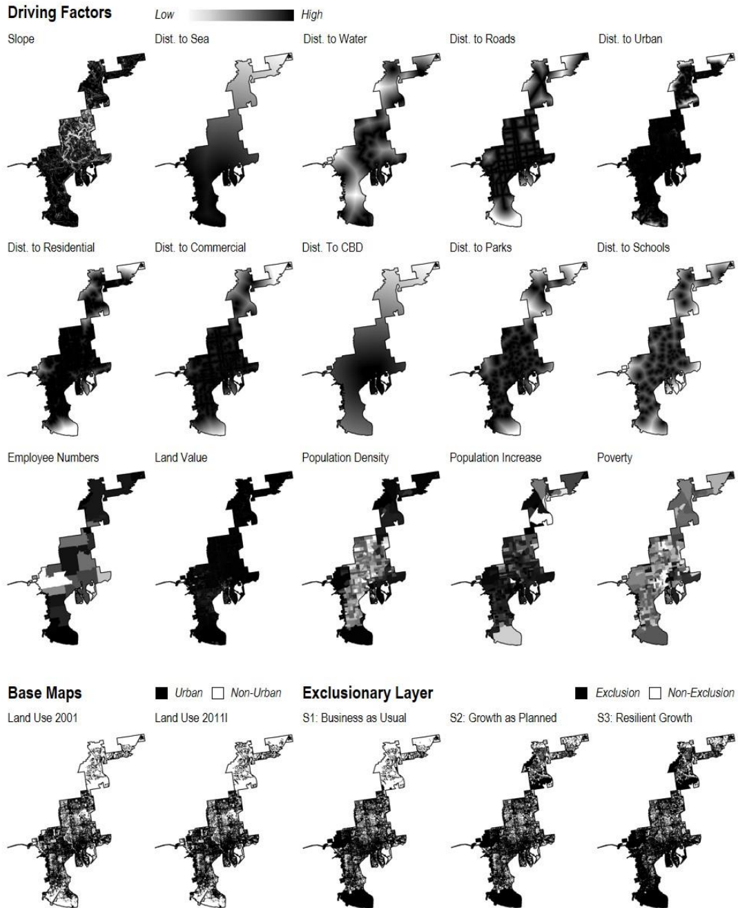
Figure A.1. Driving factors, base maps, and exclusionary layers for urban growth prediction.
