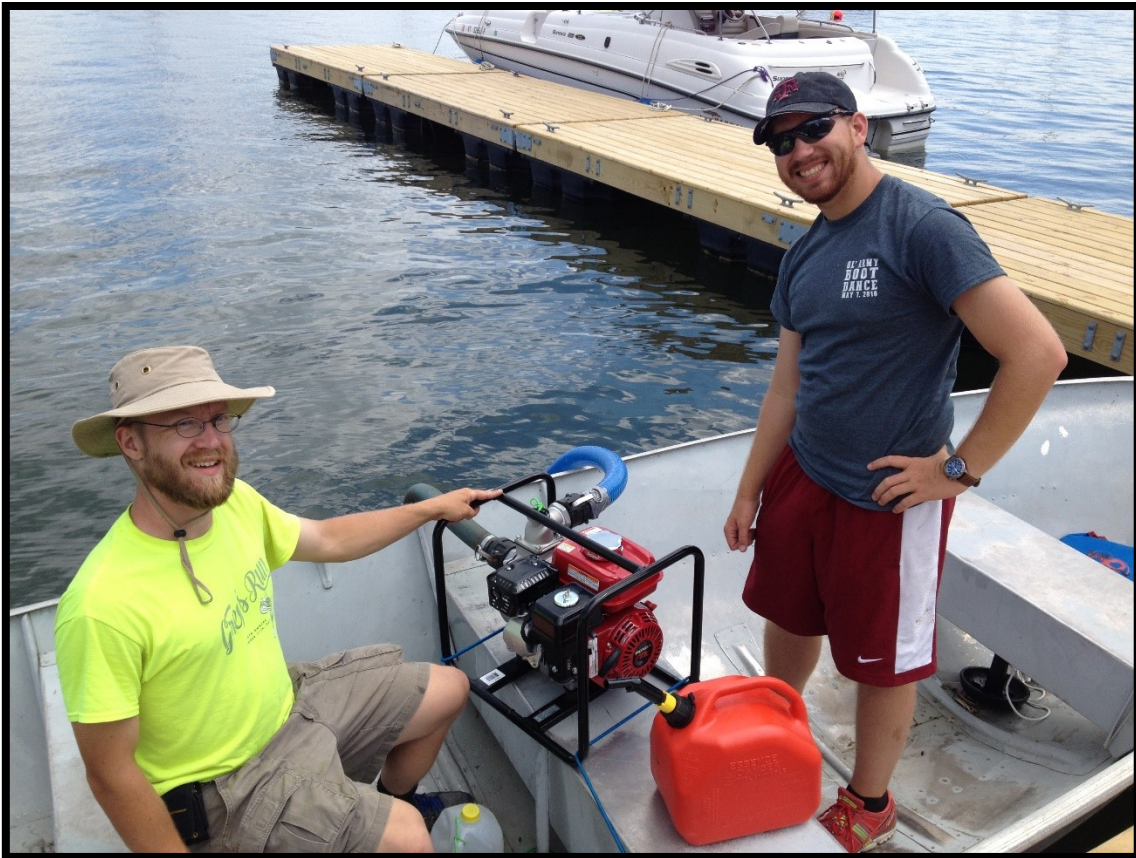
Figure 4-8. McPhee and Burford tend to the 2-inch (5-cm) Honda dredge pump in the LCMM aluminum tender. (Photograph by C. Kennedy, 2016)
