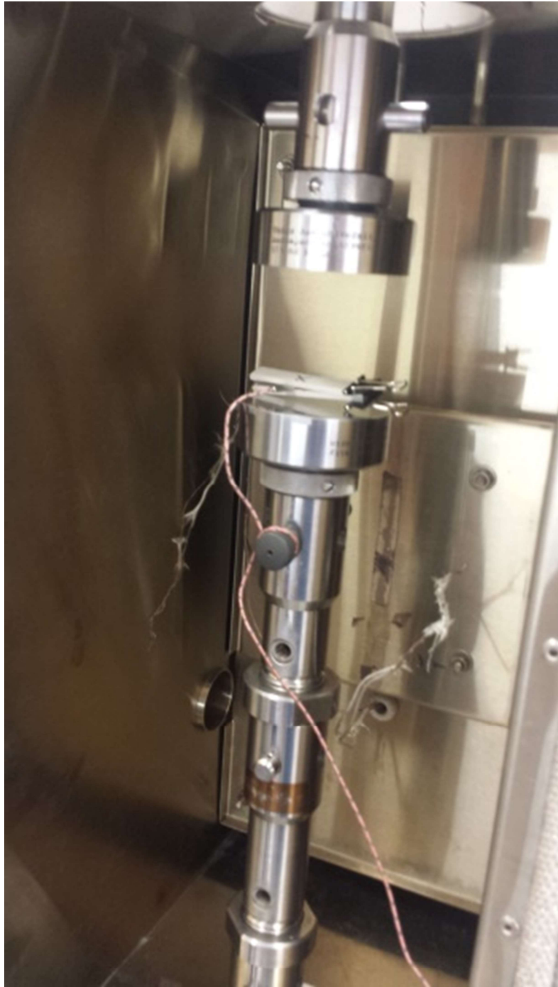
Figure 8. Specimen temperature test setup
