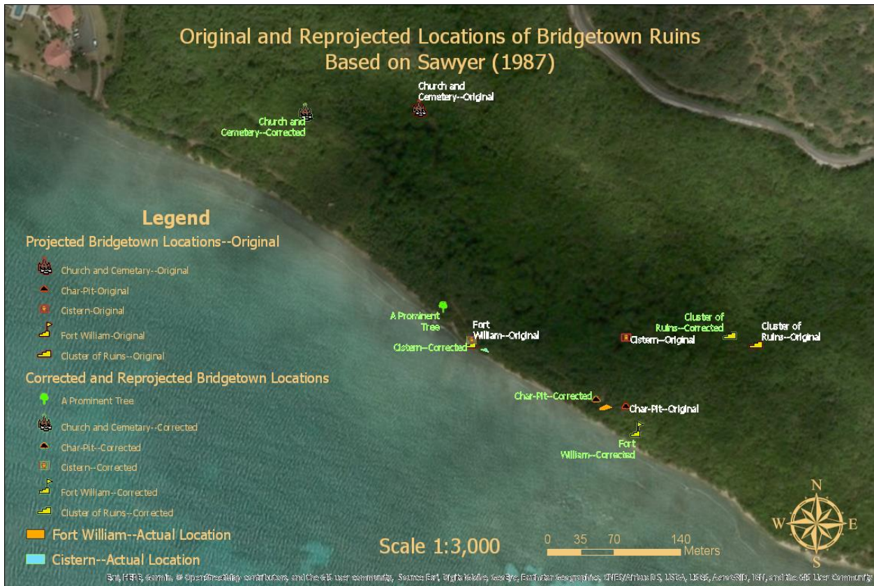
Figure 20 Original projections by Dr. Cory Look based on Sawyer (1987) and corrected locations based on survey observations and corrected map projection information.
