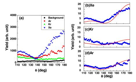
FIG. 4 (color online). (a) Experimental angular distributions for background, Ar, Kr, and Xe at  $8.3 \times 10^{13}$  W/cm<sup>2</sup>. (b)–(d) Background-subtracted and normalized angular distributions, compared to theoretical differential cross sections (in a.u.) for backscattering of 14.4 eV free electrons ( $p_0 = 1.03$  a.u.).
