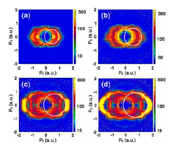
FIG. 2 (color online). Density plots of electron momentum spectra at different laser intensities for 7 fs pulses on Xe. The intensities (in units of  $10^{13}$  W/cm<sup>2</sup>) and corresponding values of  $p_0$  (in a.u.) are, respectively, (a) 4.18, 0.74; (b) 5.8, 0.86; (c) 7.1, 0.95; (d) 8.3, 1.03. The white circles show the inner edges of the regions from which the differential cross sections were extracted (see text).
