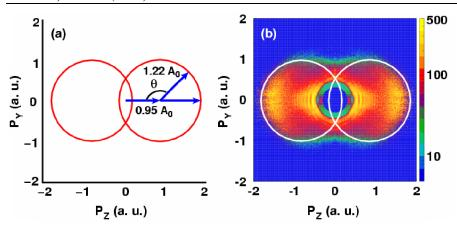
FIG. 1 (color online). (a) Schematic showing the relative sizes of the momentum vector of a returning electron with maximal energy and the momentum shift which this electron will receive from the laser field after recollision, at  $8.3 \times 10^{13} \text{ W/cm}^2$ . (b) Experimental electron momentum image from a 7 fs pulse of this intensity on the background gas of water vapor and hydrocarbons.
