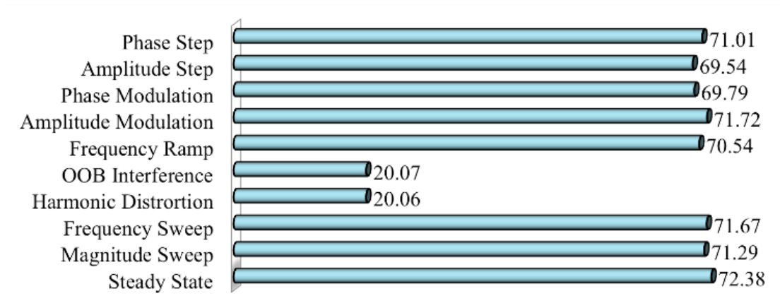
Figure 9. Signal to noise distortion ratio (SINAD) (dB) over the set of type tests defined in the IEEE standard for M-class PMUs.
