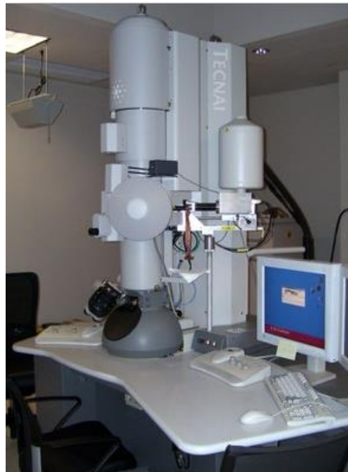
Figure 2.14 A photo of FEI Tecnai G2 F20 ST FE-TEM in MIC at Texas A&M.
