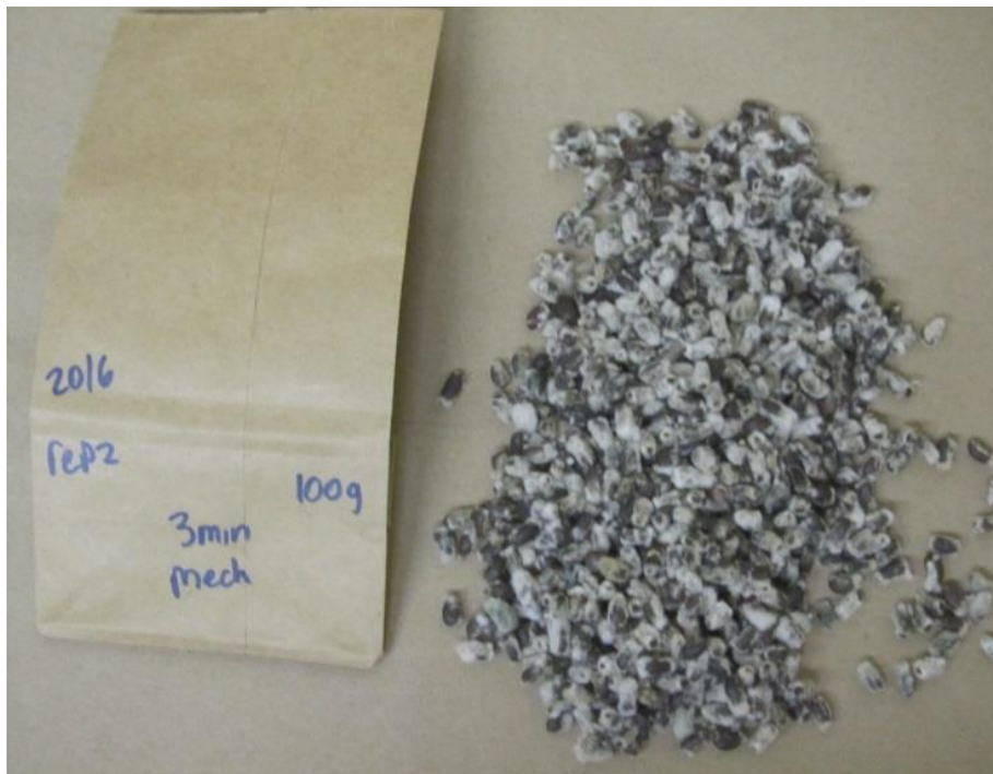
Figure 19. Delinted cottonseed from a 100 g sample delinted with a mechanical cottonseed delinter for 3 min from the 2016 timed weight experiment.
