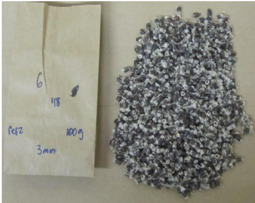
Figure 20. Delinted cottonseed from a 100 g sample delinted with a mechanical cottonseed delinter for 3 min from the 2018 timed weight experiment.
