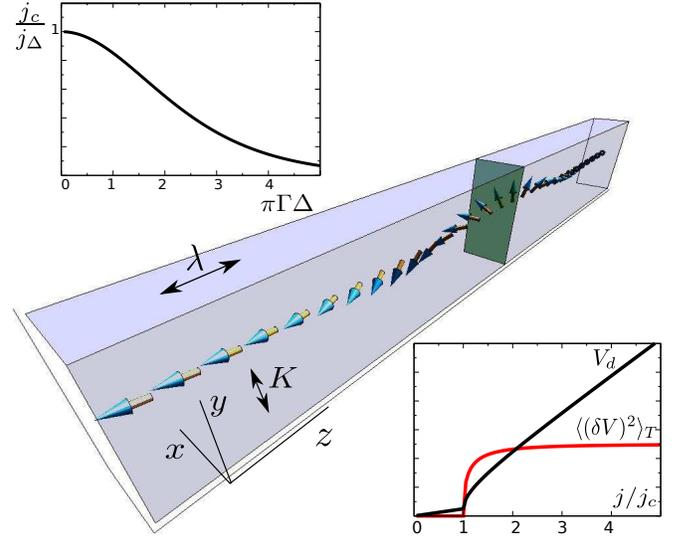
FIG. 1: (color online) Sketch of the wire with magnetization profile for a DW.  $\lambda$  and  $K$  denote the anisotropies along and transverse to the wire, respectively. The upper inset shows the dependence of  $j_c$  on the twist  $\Gamma\Delta$ , Eq. (18); the lower inset shows drift velocity  $V_d$  and variance  $\langle (\delta V)^2 \rangle_T$  (in arb. units) vs. current  $j$ , see Eqs. (20) and (21).
