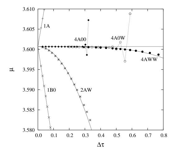
FIG. 2: The convergence of fourth-order algorithms in computing the chemical potential of the Gross-Pitaevskii equation in a rotating trap. Algorithms 4A00 (solid diamonds) and 4A0W (circles) are unstable beyond  $\Delta \tau \approx 0.3$  and 0.45 respectively. Algorithm 4AWW (solid circles) is stable and showed excellent fourth order convergence.
