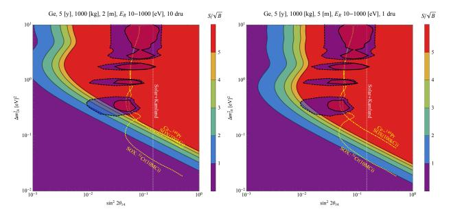
FIG. 4: Phase-2 prospective limit of  $\nu_e - \nu_s$  mixing parameters with 1000 kg Ge detector mass and 5 year effective exposure at a sample distance of 2 m (left) or 5 m (right) from the reactor. A minimum recoil threshold of 10 eV is adopted. The additional background component is modeled with a strength of 10 or 1 dru at the near and far positions, respectively. Contours and overlays are as described in FIGS. 3.
