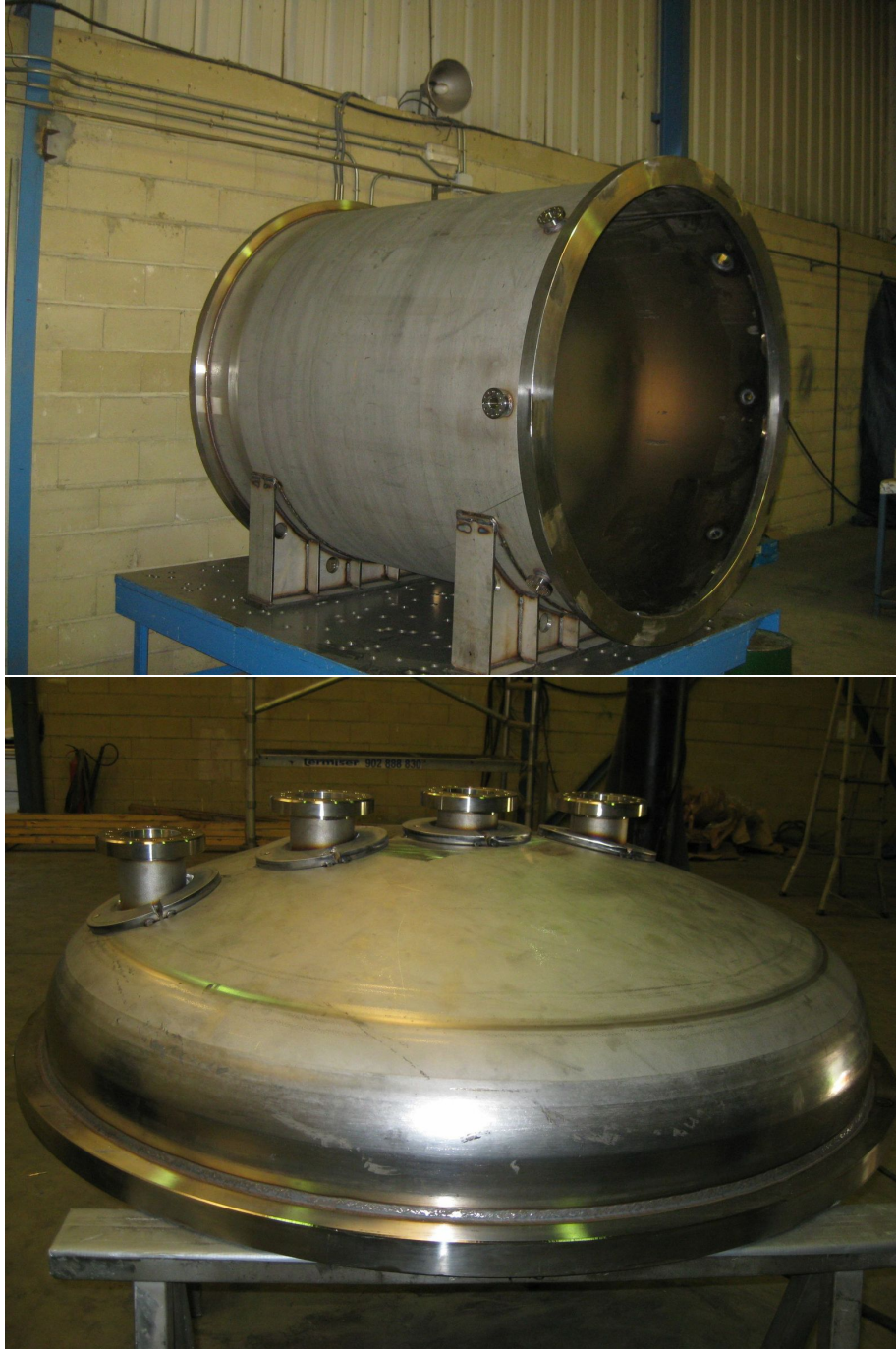
Figure 8. NEXT-100 vessel in the finale stages of the production. Main body of the vessel (top), endcap with the port to extract the different signals and circulate the gas (bottom).
