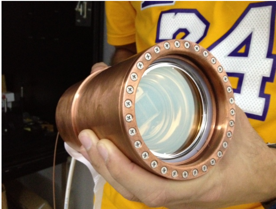
Figure 12. The pressure-resistant enclosure, or “can” protecting the PMTs inside the PV.
