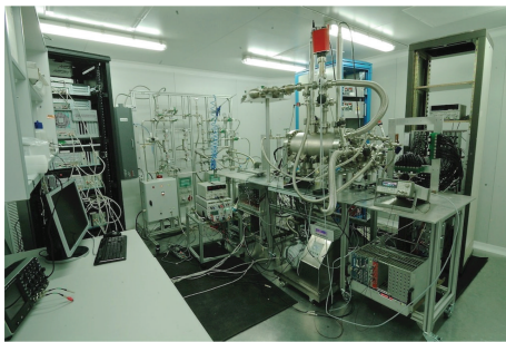
FIGURE 21: The NEXT-DEMO detector and ancillary systems (gas system, front-end electronics, and DAQ) in their location in the operation room at IFIC.
