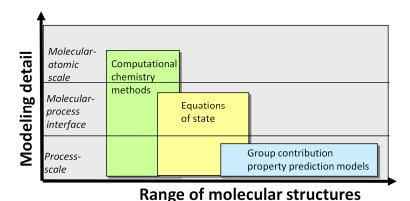
**Figure 2.** Property prediction models with respect to modeling detail and range of molecular structures which may be simulated at a reasonable computational effort.
