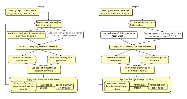
**Figure 4.** Algorithmic steps involved in the optimization-based CAMD approach for simultaneous mixture and ORC design used in Papadopoulos *et al.* [18,19].
