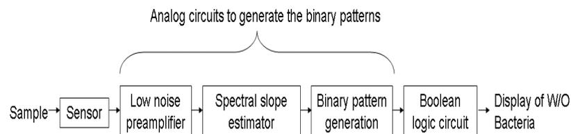
In Figure 3, the outline of the Analog Unit is shown. The preamplifier amplifies the stochastic component of sensor signal. The spectral slope estimator is the combination of a small number of amplifiers, filters and rectifiers. The binary patterns are generated by a set of comparators.
