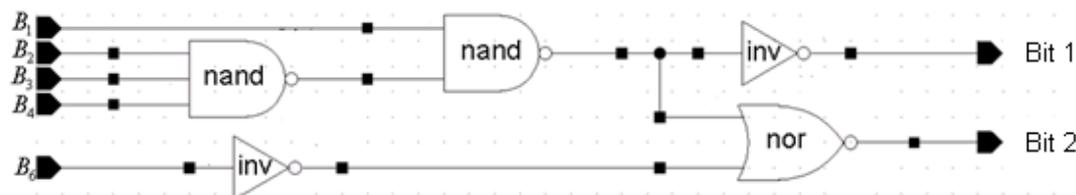
When this Boolean logic circuit is realized by CMOS logic gates, its static power consumption is in the nano/picoWatt regime. In addition, this circuit consumes some extra power for a short time (nanosecond) while it switches when the situation of agents change. Due to the rarity of such events, the power consumption in the Binary logic is basically due to the leakage current of transistors. At practical situations, these powers required by the logic circuitry are negligible.
