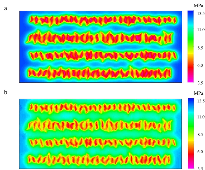
Figure 7. Pressure distribution of the non-planar fractures case at the end of 30-year production with and without the capillary pressure effect. (a) Without the capillary pressure effect; (b) With the capillary pressure effect.
