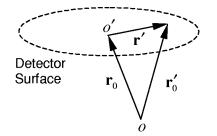
FIG. 3. Diagram of the detector surface  $\mathbf{r}'$  with origin o'. The vector  $\mathbf{r}_0$  represents the center of detector o' in the recording geometry with origin o. The vector  $\mathbf{r}'_0$  points to an element of the detector aperture.
