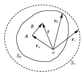
FIG. 1. Diagram of the recording geometry: a recording surface  $S_1$  completely encloses another recording surface  $S_0$ ; there is a point source A at  $\mathbf{r}_a$  inside  $S_0$ ; R is the distance between an arbitrary point at  $\mathbf{r}$  and the point source A;  $\mathbf{r}_0$  and  $\mathbf{r}_1$  point to a detection element on the surfaces  $S_0$  and  $S_1$ , respectively.
