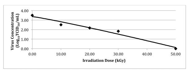
Fig 2. Inactivation of PEDV by eBeam irradiation processing. Inactivation curve modeled by the Weibull model for the survival of PEDV in complete feed when exposed to eBeam irradiation.
