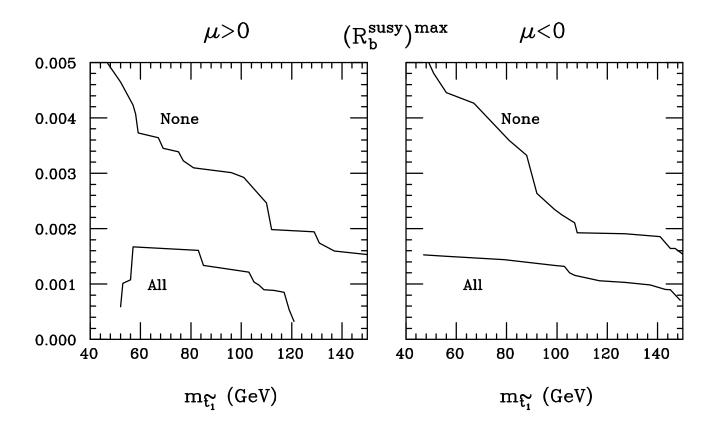
Figure 2: The maximum attainable value of  $R_b^{\text{susy}}$  versus the top-squark mass for both signs of  $\mu$ , when no constraint has been applied ("None") and when all constraints have been applied ("All"). It can be seen from this plot how the expected future direct limits on  $m_{\tilde{t}_1}$  from the Tevatron will constrain  $R_b^{\text{susy}}$  further.
