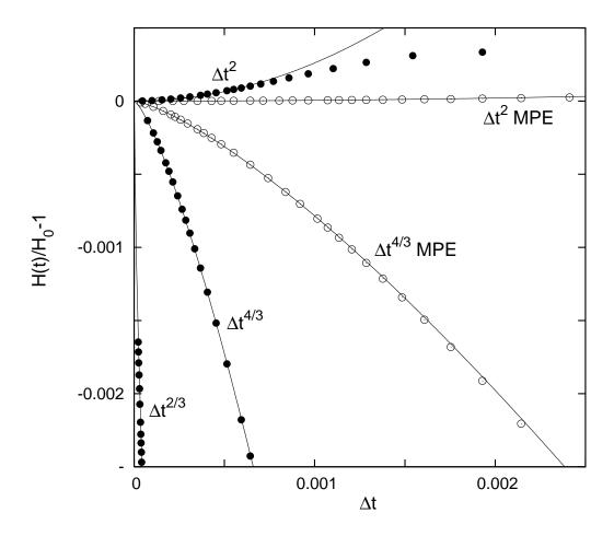
FIG. 3: The fractional power convergence of various explicit algorithms. The relative energy error is evaluated at the first quarter period t=0.385841, for the outermost trajectory of Fig.1. The solid circles denote results of symplectic algorithms (18), (30) and (31). The hallow circles give results of MPE algorithms (32) and (33). The lines are fitted cuves of the form  $c\Delta t^n$ , with n=2/3,4/3, or 2 as indicated.
