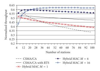
FIGURE 4: CSMA/CA versus hybird OFDMA/CSMA (M: no. of subchannels).
