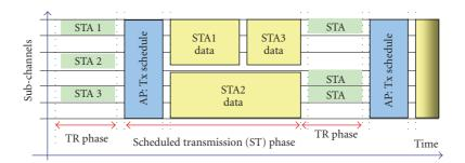
FIGURE 1: Two-phase MAC operation: TO request (TR) phase, scheduled transmission (ST) phase.
