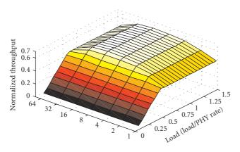
FIGURE 6: Normalized throughput versus load and number of subchannels: 32 stations throughput versus offered load.
