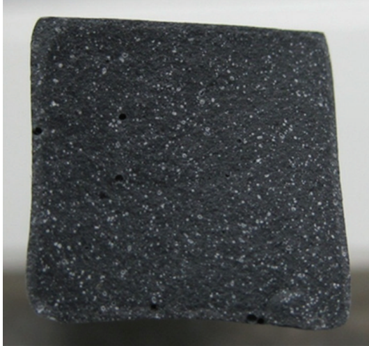
FIGURE 2: Clumps of silica fume particles (lighter colored particles) seen in the fractured surface of a hardened cement paste beam. It is postulated that these clumps generate weak zones that can partially offset the effect of CNFs on mechanical properties. The beam has a cross-section side length of 15.9 mm (0.625 inch).
