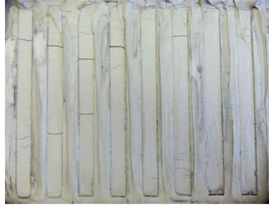
FIGURE 3: Cement paste from batch 6 ( w/c = 0.25 , without silica fume and CNF) in the molds 24 hrs after casting. The beams were exposed to drying conditions during this period and formed shrinkage cracks, some of them causing fracture through the depth of the beams before demolding. The beams have a cross-section with the side length of 15.9 mm (0.625 inch) and length of 240 mm (9.5 in).
