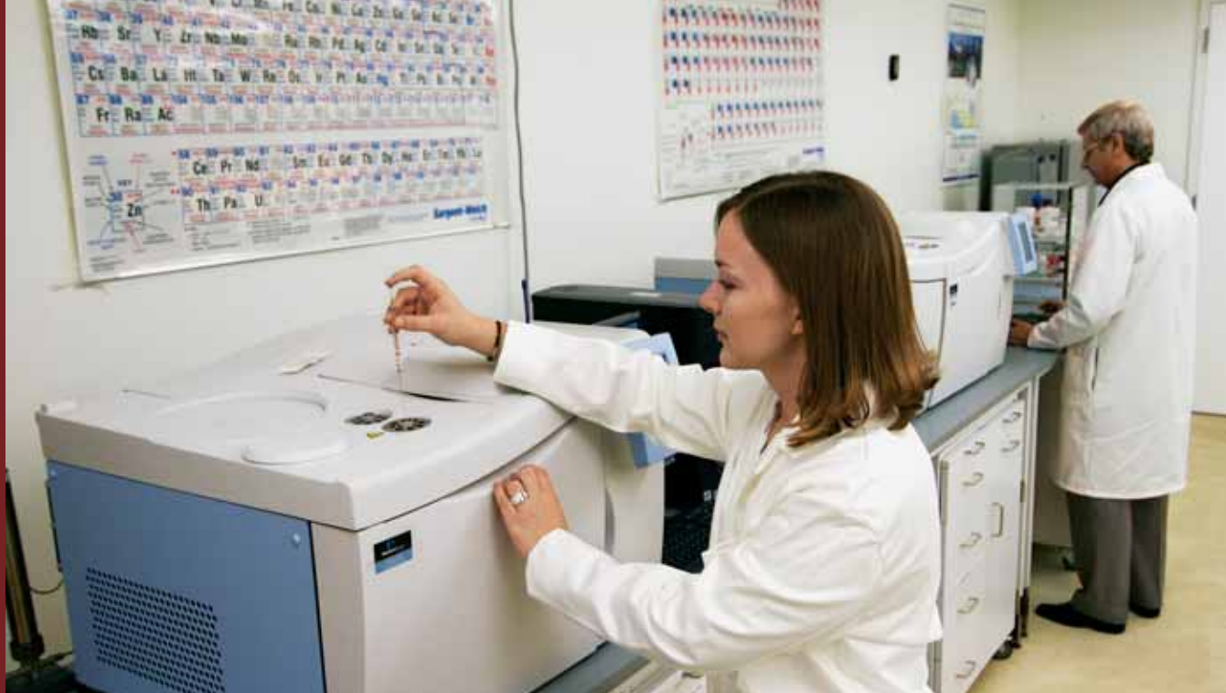
Above: Lacey Martin '05, Lab Technician, running a gas chromatograph in the TAMUQ Chemistry Lab.
