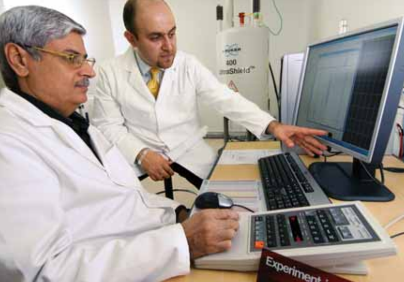
Above: Dr. Bazzi and Mr. Adel Said, Technical Lab Coordinator, looking at an NMR spectrum collected on new 400MHz Bruker magnet. Right: Dr. Bazzi inserting an NMR tube to start the first experiment on the newly installed NMR instrument.
