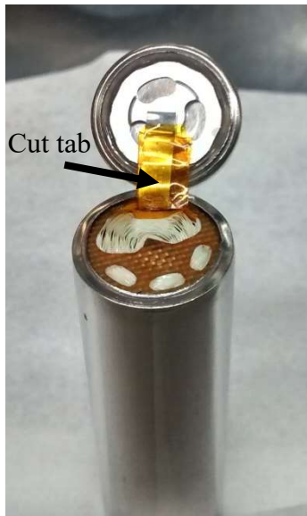
Figure 8. Cap is removed. Metal tab is cut to separate cap from case.
