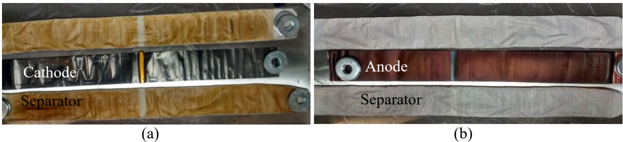
Figure 18. Electrode and separator surfaces of (a) cathode and (b) anode of externally shorted 18650 cell after performing DPA.
