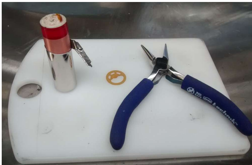
Figure 9. Aluminum case is removed by peeling it diagonally with pliers.
