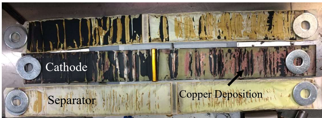
Figure 20. Center-facing cathode surface and cathode-facing separators.
