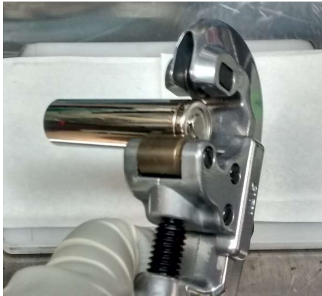
Figure 7. Cell is opened by breaking the seam with a pipe cutter.
