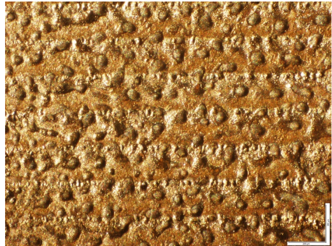
Figures 11a, 11b, 11c, 11d. (clockwise from top left) Lines at 200W & 5 Passes, Lines at 200W and 15 Passes, 5x Optical Image of Line at 200W & 5 Passes, 5x Optical Image of Line at 200W and 15 Passes
