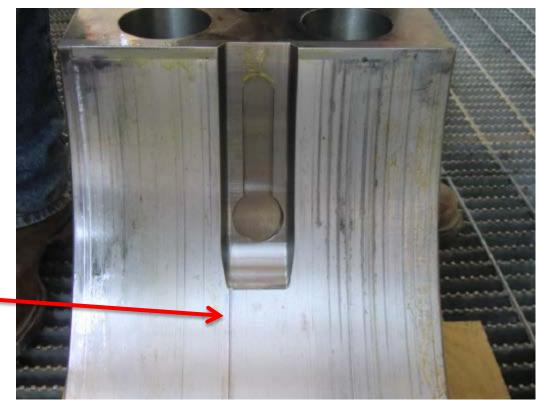
Damage due to embedded particle in shaft
