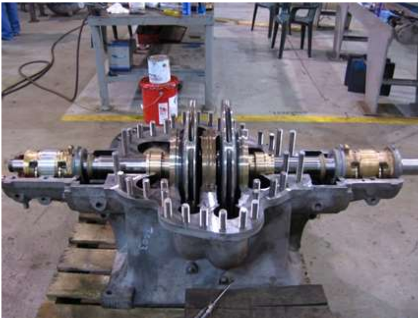
Figure 2: Axially split two-stage between-bearing process pump (Courtesy of HydroInc)
