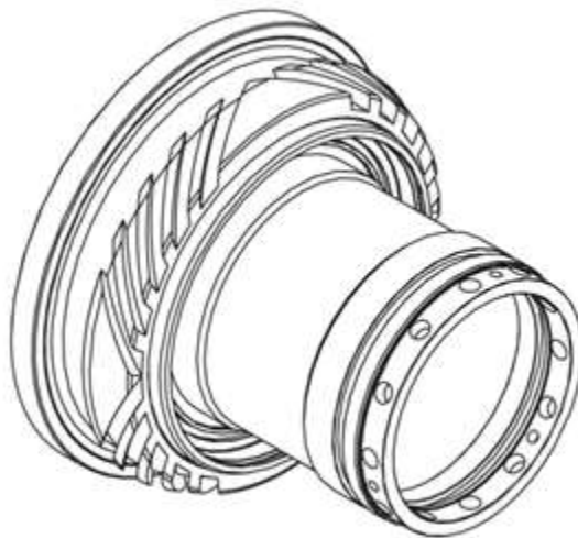
Figure 7: Bi-directional tapered pumping ring often used in dual seals for HF service (Courtesy of AESSEAL)
