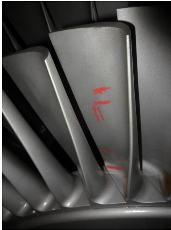
Figure 32: Stage 11 Blade with Crack to the Trailing Edge
