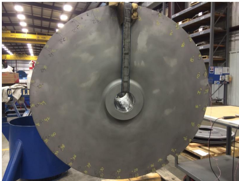
Figure 26: Impeller Impact Test Setup
