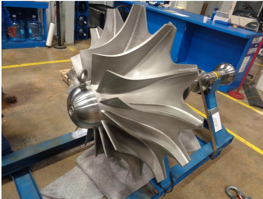
Figure 29: Impeller Geometry after Modification with “Scallops”
