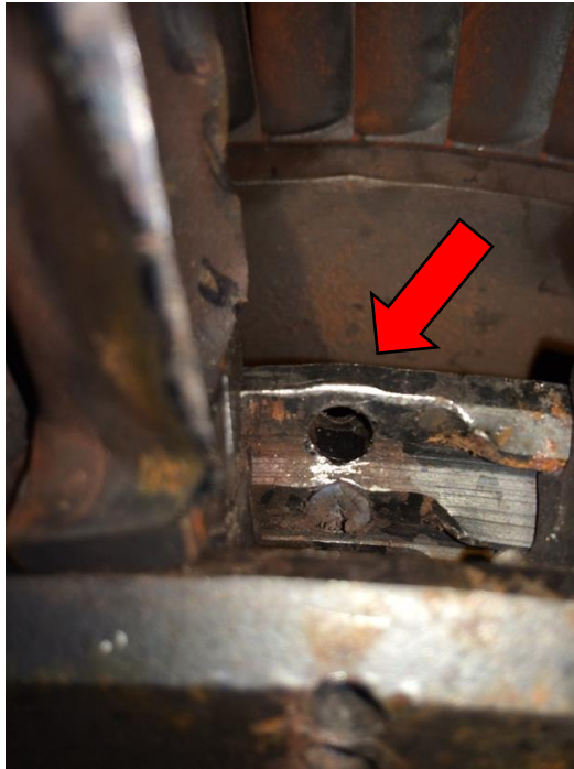
Figure 17: R-3 Locking Pin Hole Material Deformation
