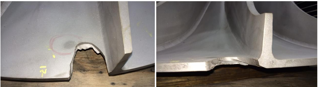
Figure 24: Backplate of the Impeller with Liberated Material Piece
