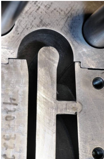
Figure 10 – Diffuser Discharging into Cast Return Bend
