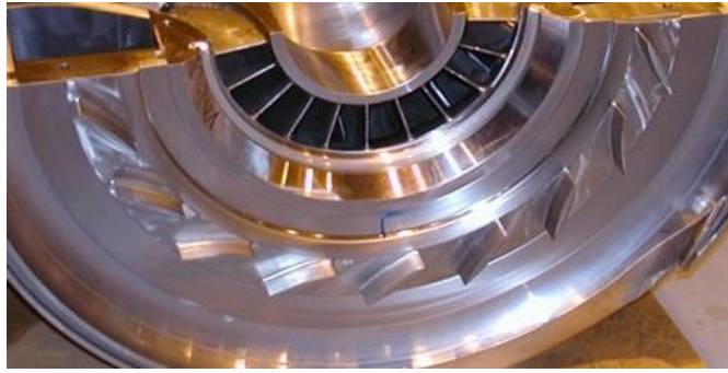
Figure 23. Low solidity diffuser vanes (LSDs)
