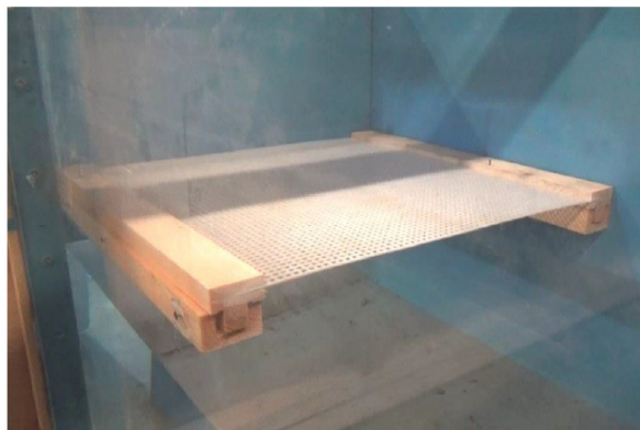
Figure 19. Anti-vortex screen over end of inlet channel.
