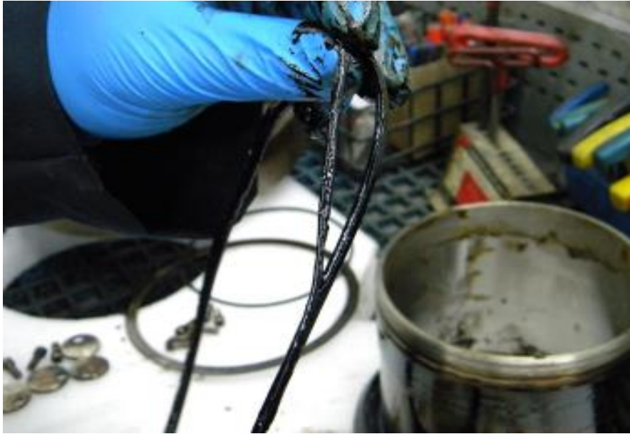
Figure 8 A typical O-ring failure due to fretting caused by pump shuttling
