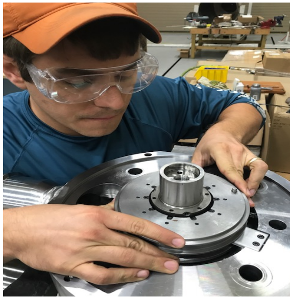
Figure 9: Turbine Assembly Showing Thrust Bearing Installation
