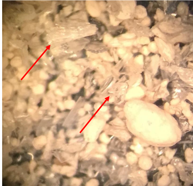
Figure 7. Site U1438 – 14HCC (127.88 mbsf). Note the abundance of volcaniclastic material (see red arrows) in the field of view. Image taken from a dissecting microscope X10 magnification.
