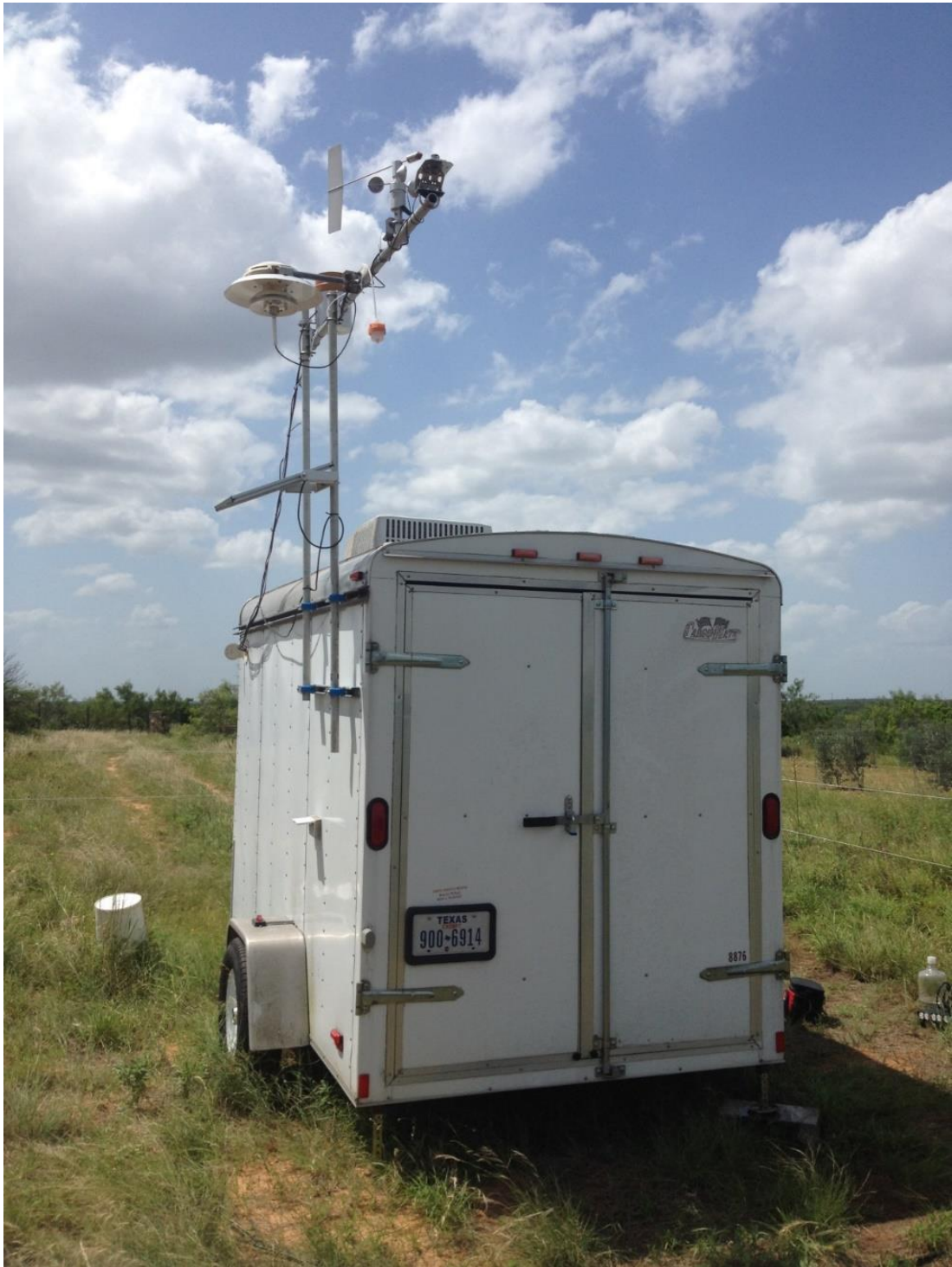
Figure 21: The trailer parked on Shape Ranch. Meteorological instrumentation and the inlet for trace gas instruments were mounted on a pole on the southeast corner of the trailer at a height of approximately 3 m.
