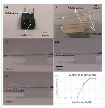
**Figure 1:** Images for smart cantilever shaped actuation material: (a) Photoimage for the 3D printed mold contained Ecoflex 30 and SMA wires. The pins as wire anchors are depicted in the picture. (b) photo-image of smart cantilever extracted from the mold. Photo-image of cantilever deflection with (c) 0, 0.5, 1, 1.5, (d) 2.0 and (e) 2.5, 3 volts application. (f) The graph for cantilever deflection angle as function of applied potential.
