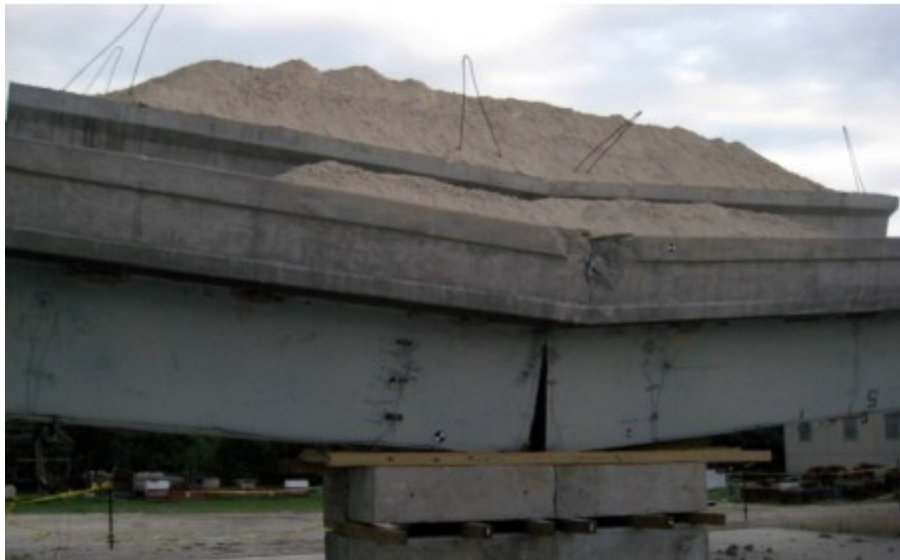
(b) Applied sand loading for full-scale testing of TxDOT 9-5498 Project
