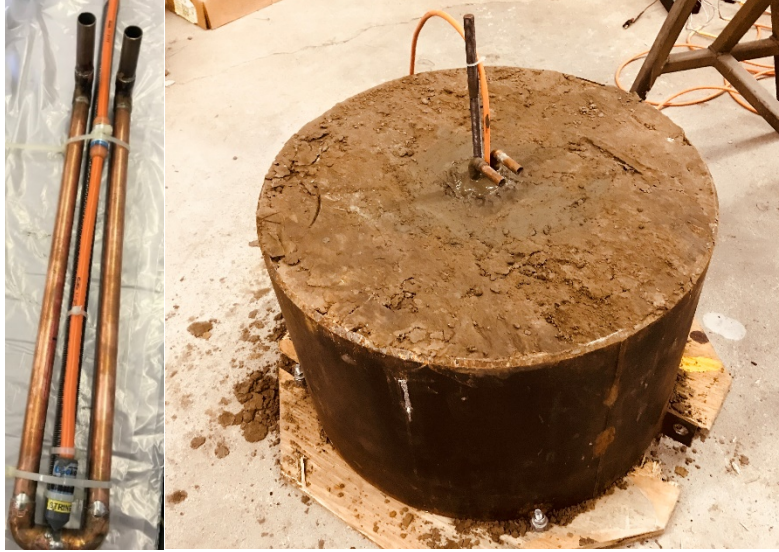
Figure 3.15. Installed the instrumented pile at the center of the sample.
