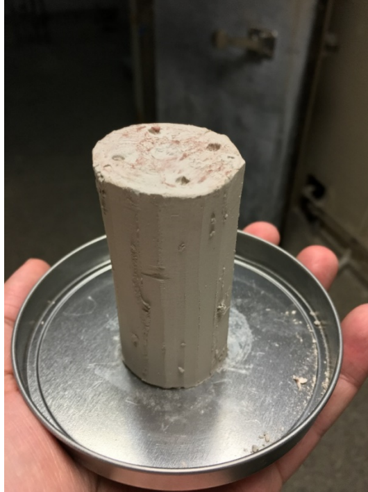
Figure 3.12. Porcelain clay sample trimmed to the dimension.
