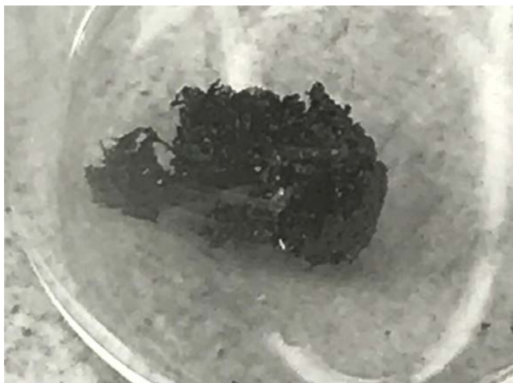
Figure IV-10. A piece of char of PMEOPC after TGA.
