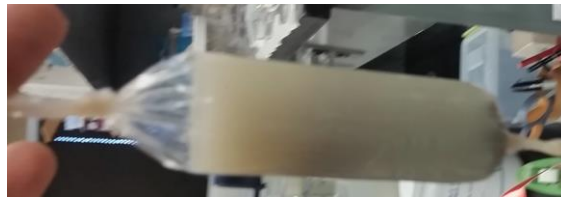
Fig. 3— Dialysis tube with clay slurry for salts wash.
