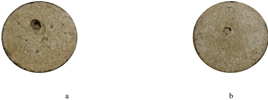
Fig. 96— Core inlet and outlet of the high-permeability core (HP-04) used in DC-02: (a) core inlet, and (b) core outlet.
