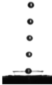
Figure 5. Droplet train imaging conducted by Zhang [1] and Muthusamy [24]. Image reprinted from Zhang [1]
