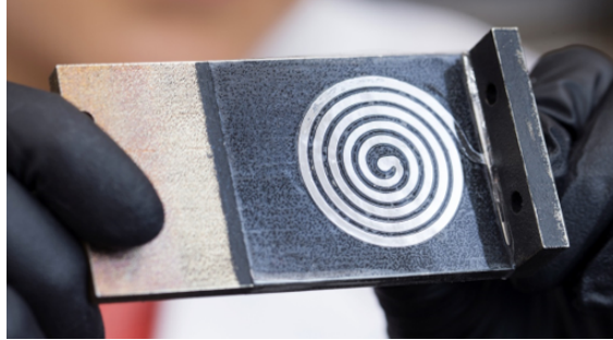
Figure 2.1: A liquid metal filled external surface channel embedded the configuration of a planar induction coil in an SMA produced via L-PBF. The black surface is a Xylan® polymer coating isolating the shiny liquid metal.
