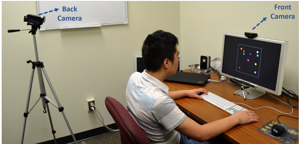
Figure 5.27: Front and back camera positions for both single and dual video threat models.
