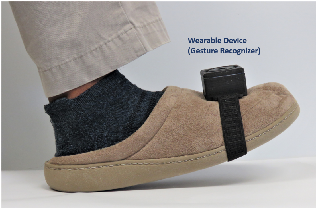
Figure 4.4: Foot Gesture Recognition Device - Master unit: the entire circuitry of the master unit is housed inside a 3D-printed container that is attached to the user's footwear. The user is executing a toe tap gesture.
