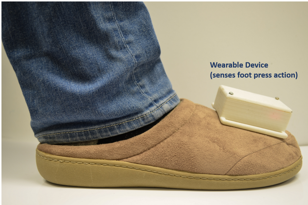
Figure 4.9: Foot Press Sensing device attached to the user's footwear. The pressure sensor is placed inside the footwear.
